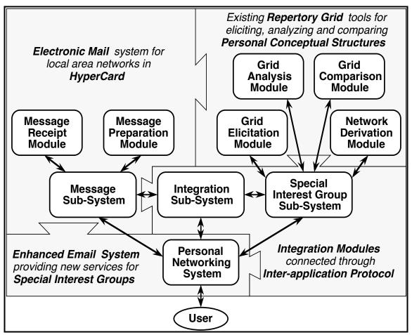
Fig.4 System architecture
