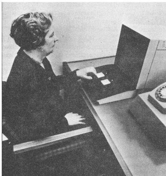
Fig. 8. Random-access microfilm terminal and reaction-time logger used in psychological assessment.
