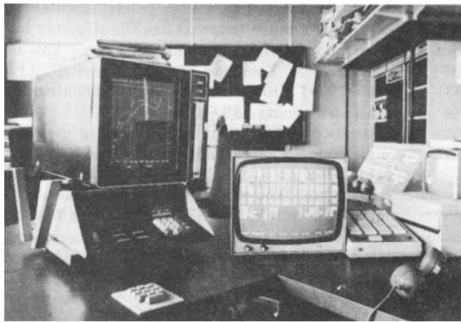
Fig. 3. Gilt-edged security dealing station in Stock Exchange office. Foreground left: graphic display and keyboards. Center: television monitor display of prices and yields. Right: telephone key system. In the right background can be seen the computer.
