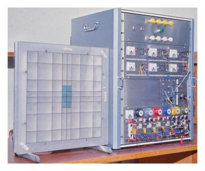
**Fig. 6** On right, stochastic analog computer designed by Brian Gaines and built by Peter Joyce; on left, visual display of STeLLA learning controller's trajectory to the specified region of state space, Standard Telecommunication Laboratories, 1965
