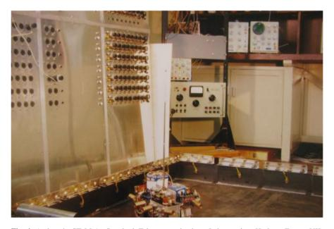
**Fig. 4** Andreae's STeLLA, Standard Telecommunications Laboratories, Harlow, Essex, UK, 1963: in the foreground, robot with its sensors in its environment; in the background, racks of electronic equipment and potentiometers for adjusting weights implementing the learning algorithms
